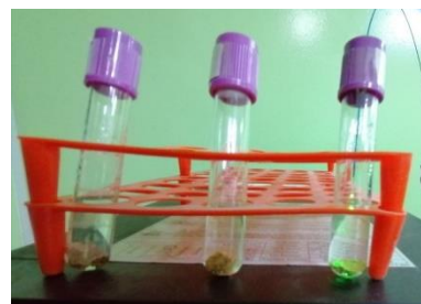
Image 4: The samples of irradiated stone after exposure to Ho-YAG laser represent different energies.
