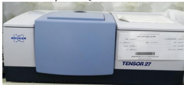
Image 3: Bruker FTIR-Spectrometer device and using a potassium bromide tablet at University of Thi-Qar/ College of Science/Department of Chemistry.
