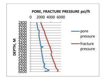
Fig. (5): pore pressure and cracking pressure versus depth (first way calculating)
