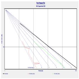
Fig. (4): Chart for pore pressure and cracking pressure versus depth
