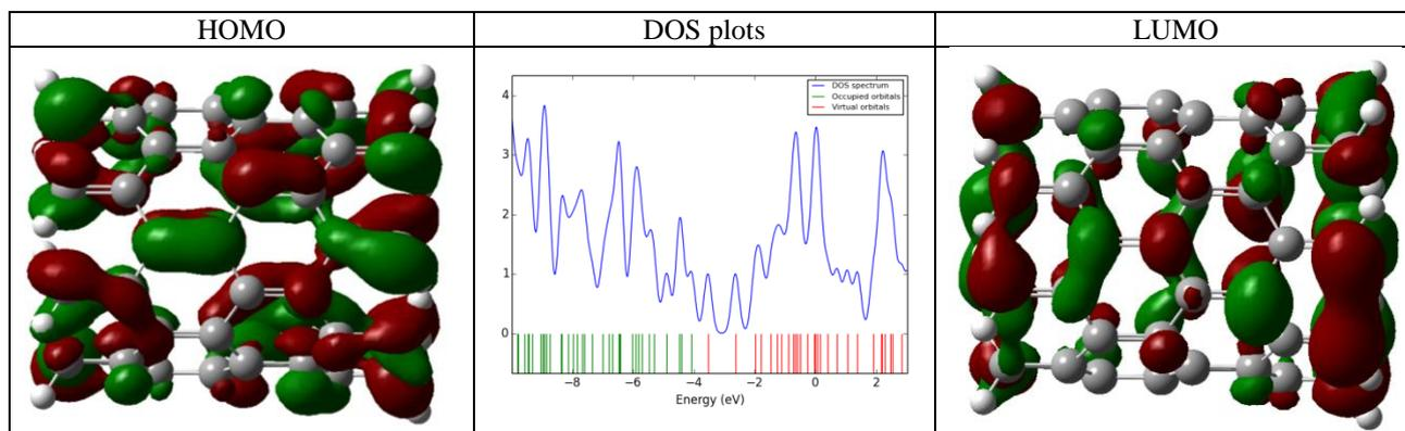
Fig.2. The density of states as well as HOMO – LUMO distribution of carbon nanotube
