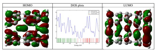
Fig.2. The density of states as well as HOMO - LUMO distribution of carbon nanotube
