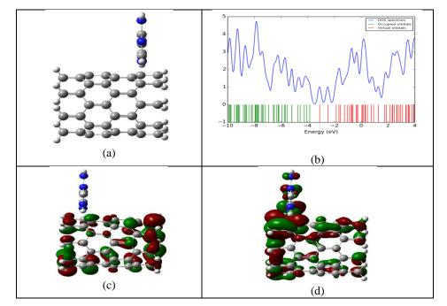
Fig. 4: a) Geometrical optimization of CNT, b) DOS, c) HOMO distribution and d) LUMO distribution
