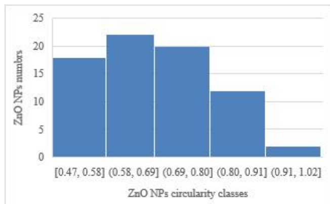
Fig. 13: Circularity distribution of green synthesized ZnO NP using Q. infectoria leaf extract, indicating shape uniformity and morphology.
