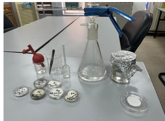
Fig. (3) : The filter device (Fakhner) used to filter polluted water.
