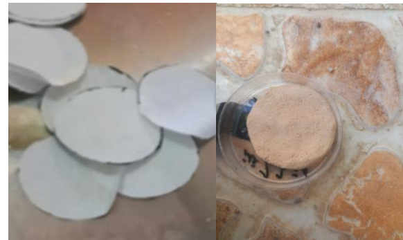
Fig. (2) : A picture of paper and clay filters used to filter water contaminated with E. coli bacteria .
