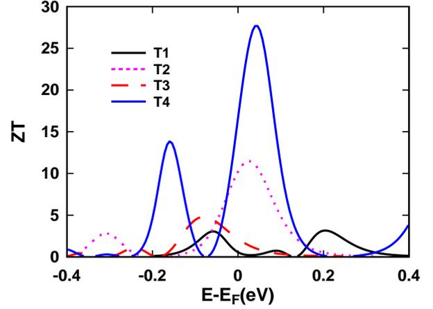
Fig.5 Thermoelectric figure of merit  $ZT$  as a function of Fermi energy for all ferrocene trimer junction.
