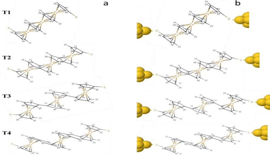
Fig.1 (a) Schematic illustration of the configuration of four trimer ferrocene structures. (b) all molecular junctions consist of ferrocene trimers sandwiched between two gold electrodes.
