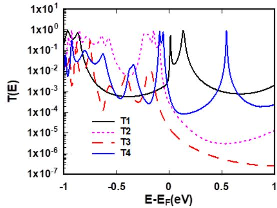
Fig.2: DFT-transmission probability,  $T(E)$ , as a function of energy for T1, T2, T3, and T4 ferrocene molecular junctions appeared in Fig.1.
