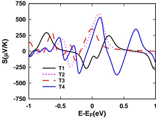
Fig.4 : Seebeck coefficient  $S$  as a function of Fermi energy for all ferrocene trimer junctions
