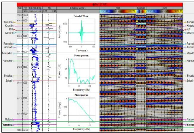
Fig. 4. Synthetic generation of well Ns-1 with to seismic line NN23.
