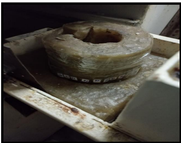
Fig. 4: 241 Am-Be neutron irradiation station
